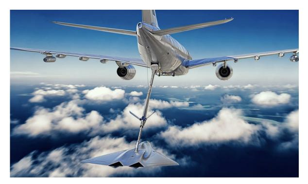
The engine air intakes are not visible, suggesting they are mounted below the airframe, something that has also been seen on previous sixth-generation concepts. It's also possible that the intakes have been omitted from the artwork entirely, to conceal the approach that Lockheed has taken here. A low-observable aircraft's intake design is among its most challenging and sensitive features.
