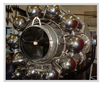
*The W2/700. The first British production jet engine which powered earlier models of the Gloster Meteor.*
