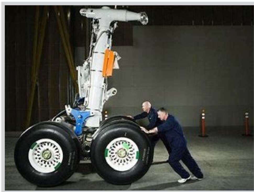
One leg of a Messier-Dowty undercarriage for a Boeing 787
