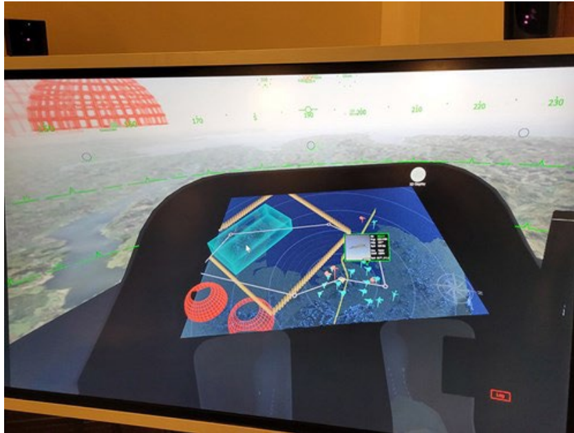
BAE Systems showed the latest version of its augmented reality fighter cockpit which now features a 3D holographic map. (Tim Robinson/RAeS)
